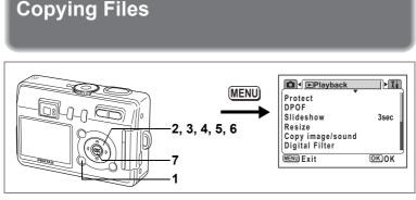
You can copy image and sound files from the built-in memory to the SD Memory Card and vice versa. This function can only be selected when a card has been inserted in the camera.
